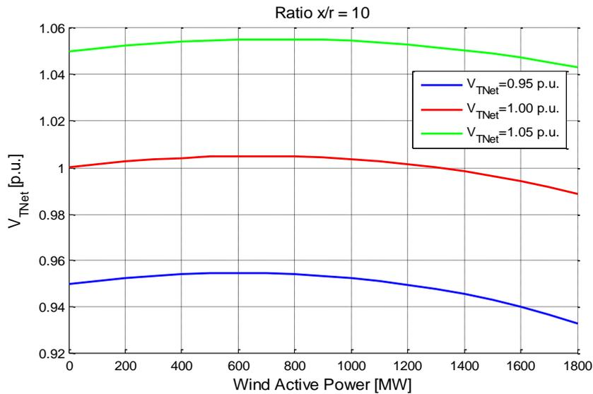
**Figure 3.5:  $V_{TNet}$  impact on the PV curve**
