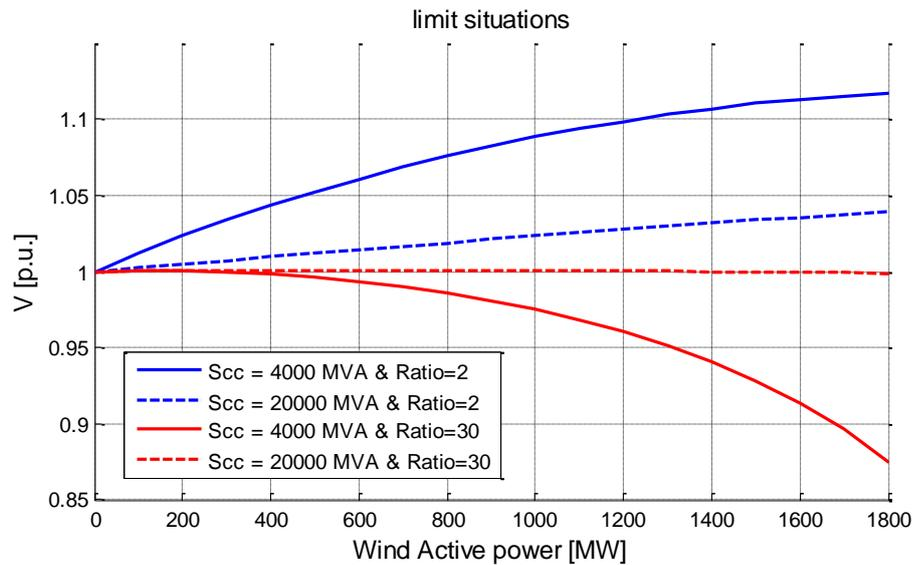
Figure 3.9: Short-circuit power (Sc) and x/r ratio impact on the PV curve
