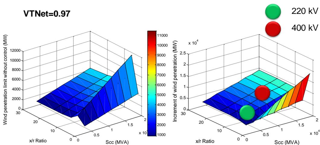
Figure 3.22: Wind penetration increment when VNet is 0.97 p.u.
