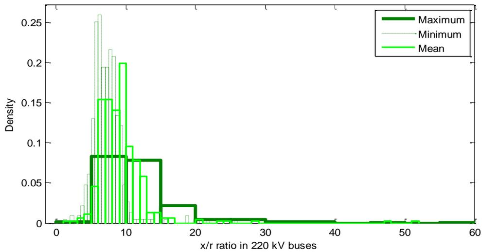
**Figure 3.19: Maximum and minimum x/r ratio in 220kV**
