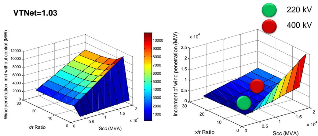
**Figure 3.24: Wind penetration increment when VTNet is 1.03 p.u.**
