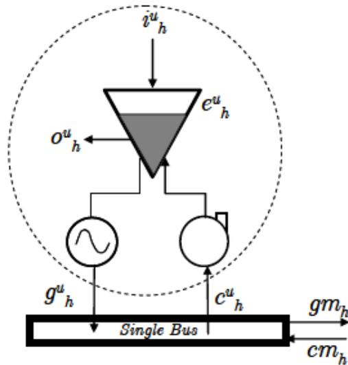
Figure 4.22: Generalized model of the VPP unit.
