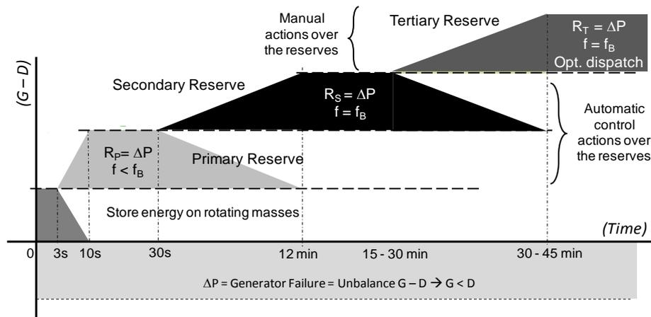
**Figure 2.1: Qualitative load frequency fundamentals and loops**
