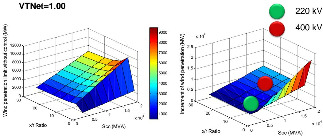
**Figure 3.23: Wind penetration increment when VTNet is 1.00 p.u.**
