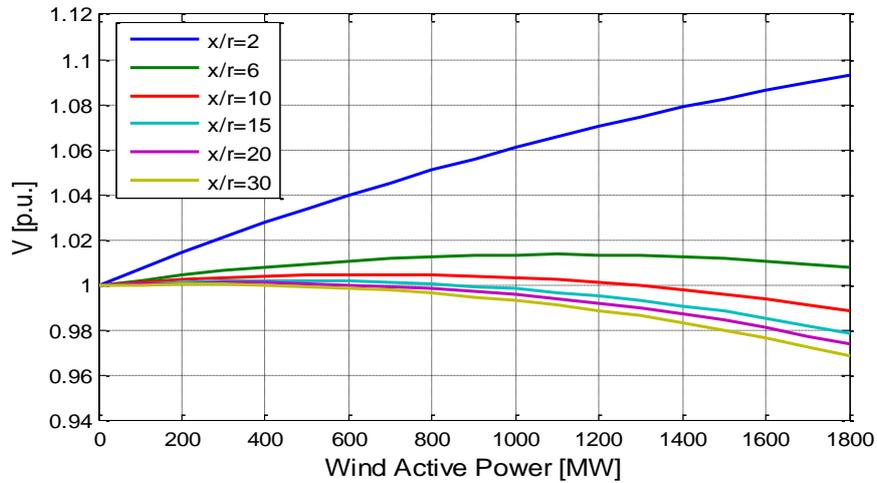
Figure 3.6:  $x/r$  ratio impact on the PV curve
