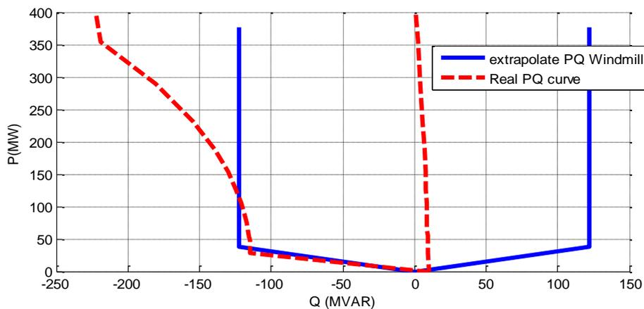
**Figure 3.29: PQ curves of the harvesting network. Taking into account the detail model of the wind farms**
